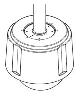
$\mbox{\#}$  To install and use OUTDOOR HOUSING, remove the Clear Case from the Camera body before installation.
